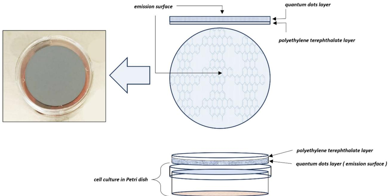
**Fig. 1** Device Assembly. It consists of a support made of Polyethylene Terephthalate (Mylar®) that is layered with graphene nanocrystals containing Quantum Dots
